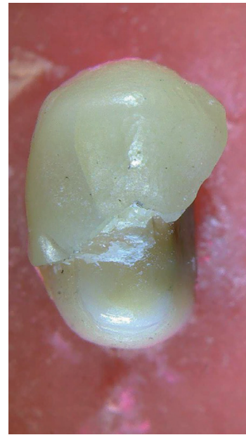
Fig. 3. Fracture of monolithic zirconia crown under a digital stereomicroscope (40×) for feather-edge margin design (Code III).
