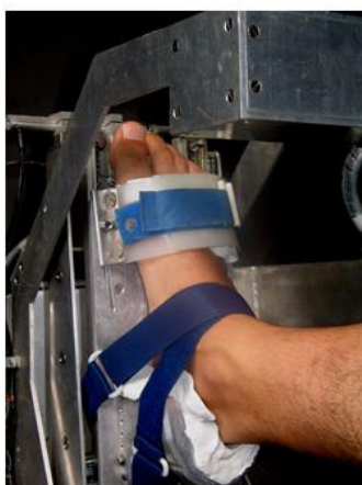
Figure 2 The ankle measurement device. A. Prototype of the ankle measurement device. B. Positioning phase of the right leg of a patient: the knee has already been fixed to the metallic fork; the forefoot has already been fixed to link 6 of the device; the rearfoot has been inserted in the ad hoc mould, and it only needs to be further fixed with Velcro stripes; the shank has already been aligned with link 0 of the device. C. Detail of a completed foot fixing.
