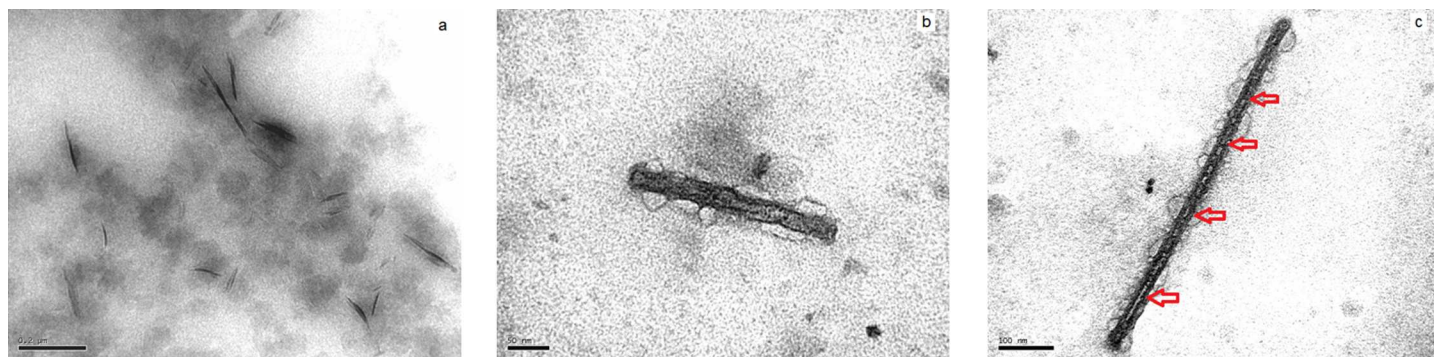
Fig 5. TEM micrographs of \alpha -LaNTs coated with silver. (a) Several nanotubes. (b) A single nanotube. (c) A silver nanotube with discontinuous silver in its lumen, the small red arrows point to silver free pockets.
