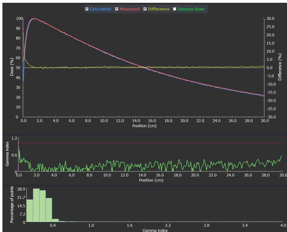
Figure 3: Comparison of simulated depth dose curve against measurements for 10 cm × 10 cm field size. The results of the gamma analysis are also shown in the figure
