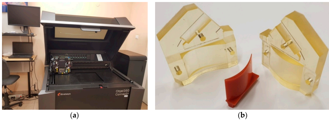
Figure 1. The process of 3D printing and wax castings; (a) Objet350 Connex 3 3D printer (b) the mold and the wax model.
