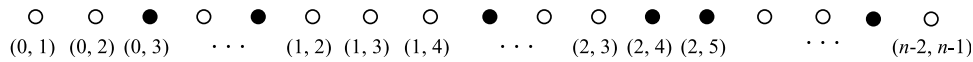
Figure 6: A sequence of all possible potential edges. Each circle represents a potential edge. The white circles are the skipped edges, and the solid black circles are the selected edges in an Erdős-Rényi graph.
