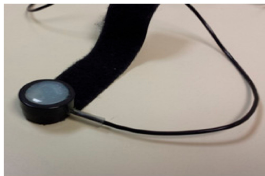
Figure 11. Piezoelectric finger sensor as a reference to determine NCVS sensor accuracy.
