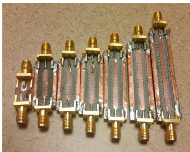
Figure 10. Example of a few phase delay modules (PDMs) used in our phased-array NCVS sensor.
