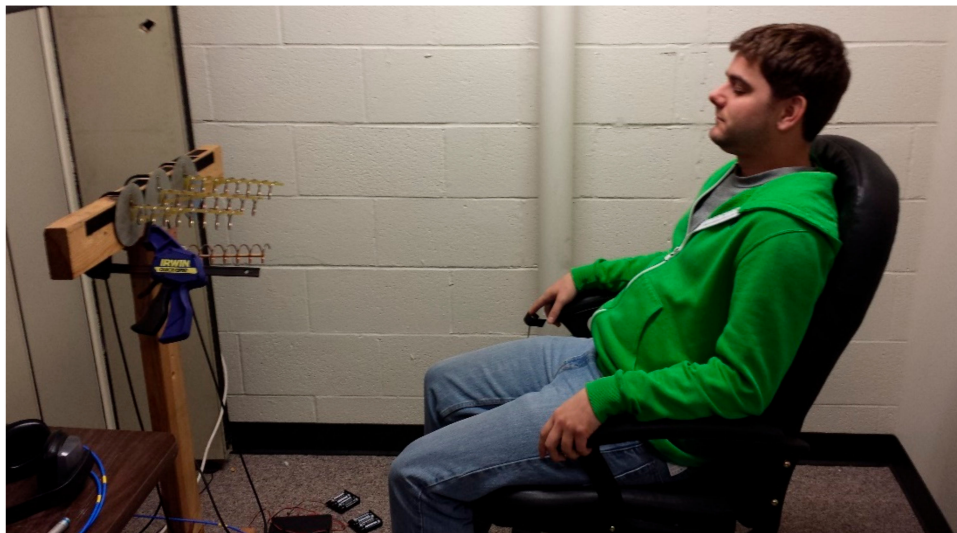
Figure 13. Subject (a student volunteer) monitored by our phased array NCVS sensor during a typical vital signs measurement setting.
