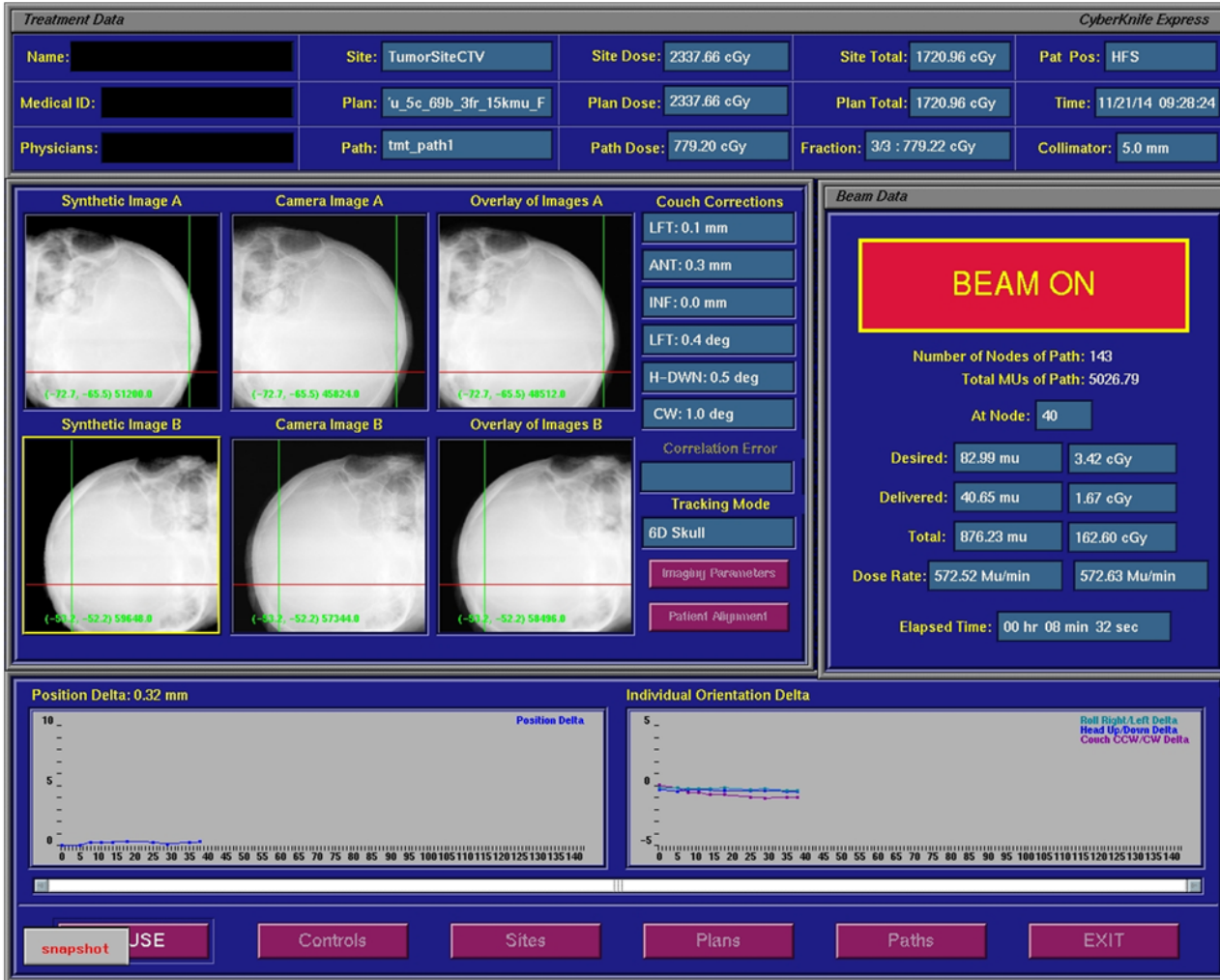
Fig 1. Image registration process. Comparison between the real time image and the DRR during radiosurgery.
