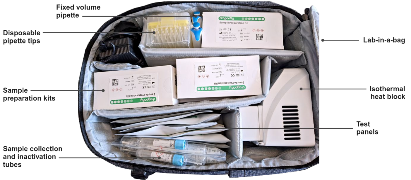
Supplementary Figure 5. Lab-in-a-bag. The entire Dragonfly platform stored in an easily portable backpack (29 x 16 x 43 cm), ready for remote deployment. Created in BioRender. Cavuto, M. (2025) https://BioRender.com/h56q657
