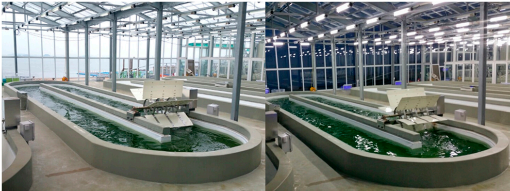
Figure 5. Photographs of the facility used for year-round cultivation of Tetraselmis sp. in six 40,000 L semi-open raceway systems (ORSs; each pond size, 12,000 (L) × 3250 (W) × 400 (D) mm; rotational speed, 15 rpm).
