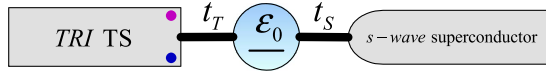
Figure 1. The junction formed by DIII -class topological and s -wave superconductors. One QD is embedded in the junction.
