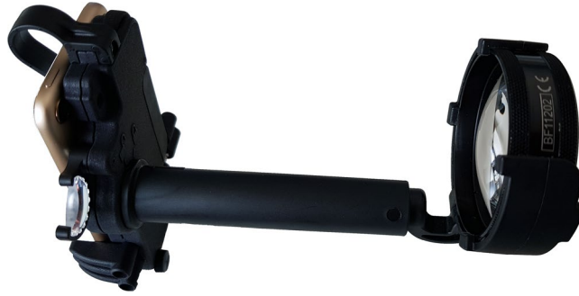
Figure 1. Smartphone-based fundus imaging device used for this study. The smartphone-based fundus imaging device was equipped with an iPod touch (sixth generation) and a Pan Retinal 2.2 for non-contact indirect smartphone-based fundus imaging.
