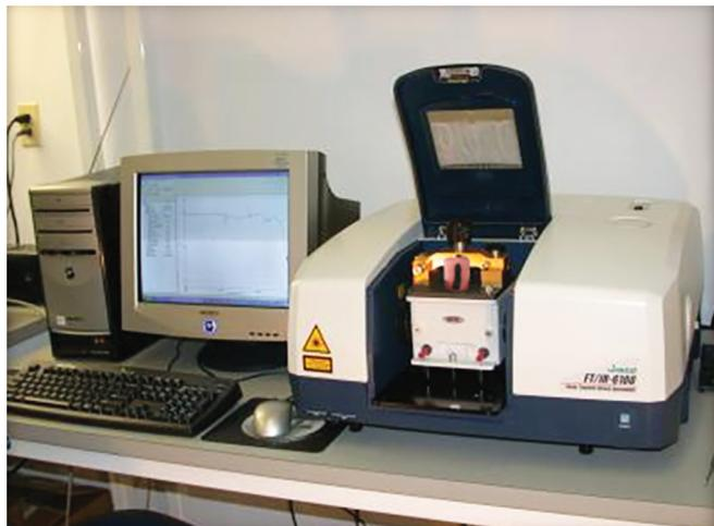
**Fig. 5:** ATR FTIR measurement
