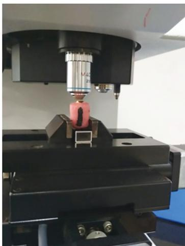
Fig. 1: Pretreatment hardness using Vickers microhardness tester
