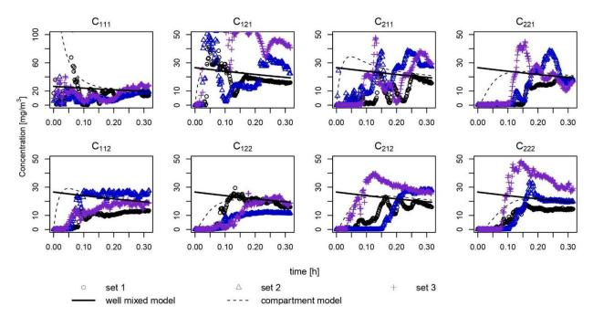
**Figure 2.** Simulation of a trigger spray containing 50% ethanol solution in the room chamber. The concentration of each compartment was measured in real-time. The scan speed of the instrument was 100 ms (millisecond).
