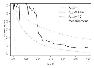
**Figure 3.** Coefficient of variation (CV) by time using the eight-compartment measurement data in a room-sized chamber (black line) and R simulation (blue lines).  $\lambda$  is the total air flow rate (h<sup>-1</sup>) and  $\lambda_{ex}$  is the air exchange rate between the adjacent compartments (h<sup>-1</sup>). The CV line at  $\lambda_{ex}/\lambda$  is 4.64 is when  $\lambda_{ex}$  was fitted with the triplicate measurement data.
