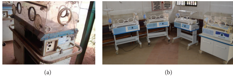
FIGURE 1: Incubators. (a) Casing recovered from a hospital dump site for recycling. (b) A fleet of recycled systems just before commissioning at FMC Lokoja.
