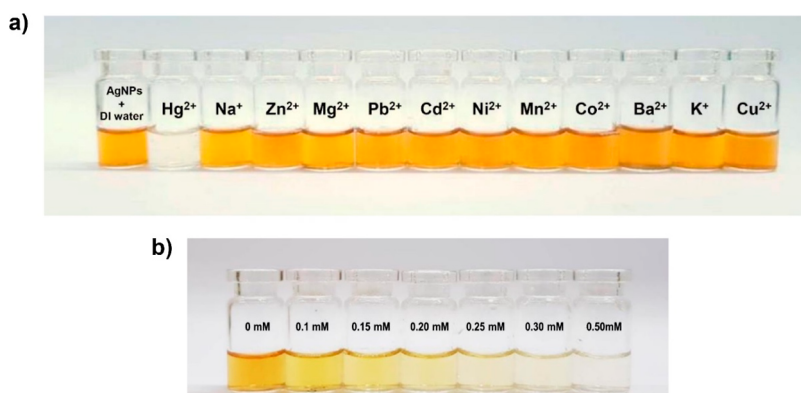
Figure 6. (a) Comparison of colorimetric responses for 0.08 nM andro-AgNPs in the presence of 20 \mu\text{M} of various metal ions. (b) Colorimetric response to different concentrations of \text{Hg}^{2+} (from left to right: 0, 0.1, 0.15, 0.20, 0.25, 0.30, and 0.50 mM).
