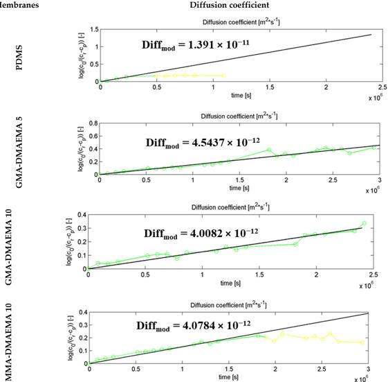
Figure 8. Experimental (linked point) and theoretical (line) diffusion coefficient of tramadol during the pertraction process with bare and modified PDMS membranes.
