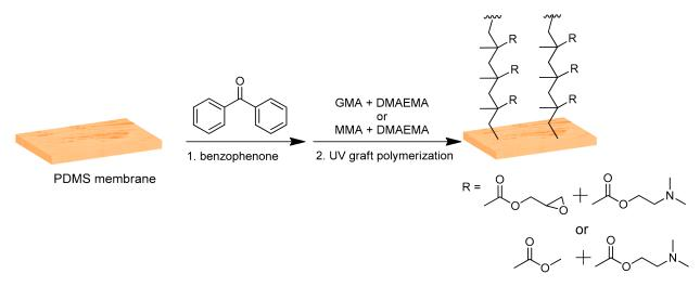
**Figure 1.** Ultra-violet grafting of polydimethylsiloxane membranes with the monomers glycidyl methacrylate or methyl methacrylate with 2-(dimethylamino)ethyl methacrylate.
