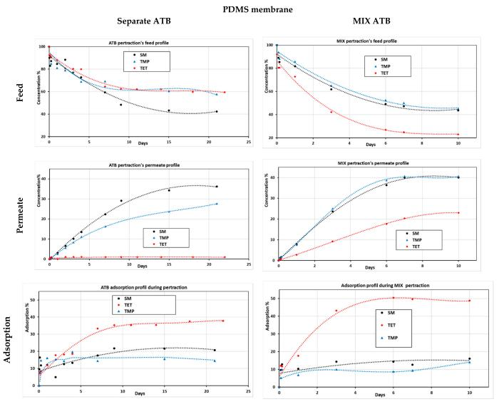
**Figure 6.** Adsorption, permeate, and feed profiles of both mixed and separated antibiotic solutions (sulfamethoxazole, trimethoprim, and tetracycline) of the pertraction process with a bare PDMS membrane.
