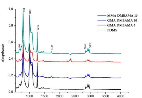
Figure 4. Fourier transform infrared spectra of bare and modified PDMS membranes on an active surface.
