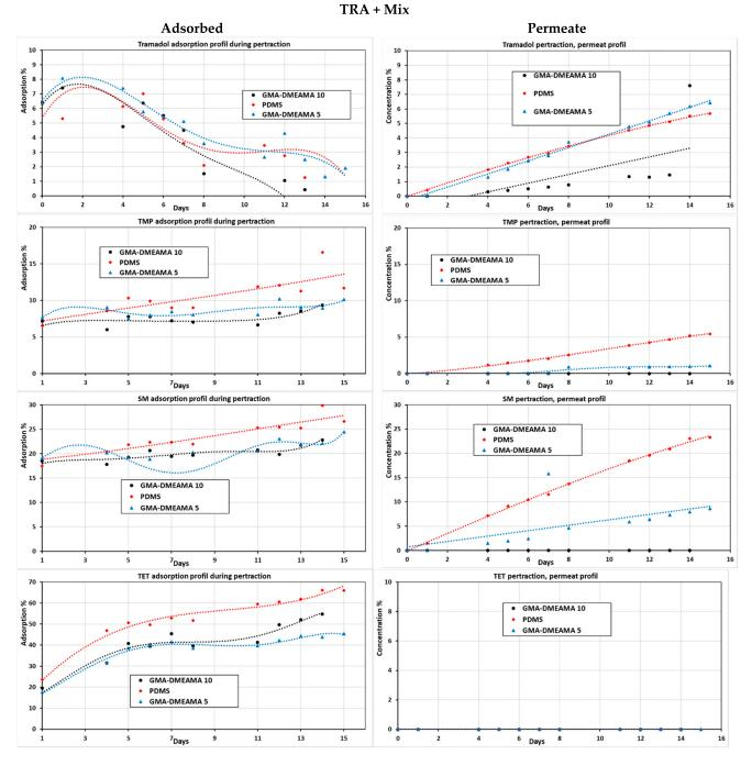
**Figure 9.** Adsorption and permeate profiles of tramadol, trimethoprim, sulfamethoxazole, and tetracycline together in the model solution of the pertraction process with bare and GMA-DMAEMA-modified PDMS membranes.
