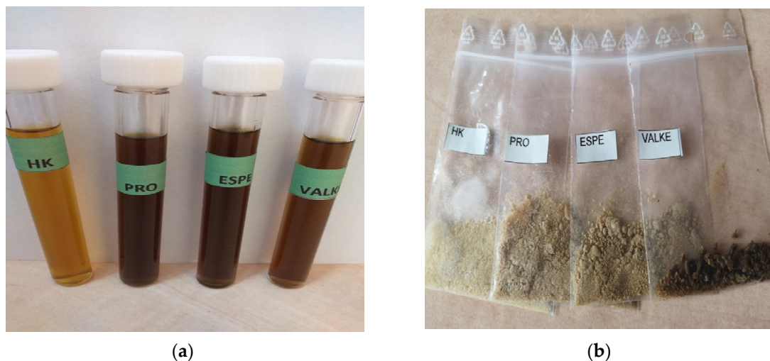
Figure 1. (a) Alkaline (HK) and enzymatic keratin hydrolysates (PRO, ESPE, VALKE); (b) lyophilised keratin hydrolysates (HK, PRO, ESPE, VALKE).
