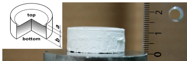
Figure 1. Non-pressed sediment sample right after demolding. The scale to the right is a centimeter-scale with each dash representing a length of 1 mm. The sample shown here has a height of 11 mm but the sample height could be scaled by changing the particle concentration in suspension or the filled height of the sedimentation vessel. The schematic on the left indicates typical dimensional and structural characteristics of our sediments: All sediments exhibit a meniscus of height a on a cylindrical body with a thickness b . For X-ray analysis, only top sections of thicknesses up to 2 mm were used. Furthermore, the schematic illustrates the distribution of polymer inside the sediments with higher fractions towards the top (darker grey) and lower fractions toward the bottom (light grey).
