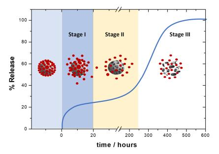
**Figure 4.** Representative release profile for polymeric NPs. In stage I the drug is quickly released through desorption–diffusion processes. The release of the drug in stage II is governed by diffusion through the polymer matrix or pores. Stage III is governed by the erosion of the polymeric matrix.
