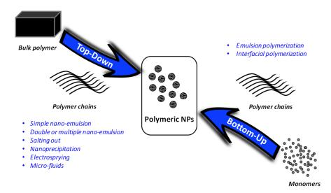
**Figure 6.** The methods to formulate polymeric NPs are divided into top-down and bottom-up methodologies. Top-down methodologies generate the NPs from preformed polymers, whereas in bottom-up methodologies the polymerization of the monomers is achieved during formulation.
