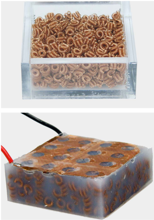
Figure 1. Photograph of a sample cell packing (top) and composite (bottom). The cell-packing forms the internal skeleton of the composite. Pouring and curing a polymeric mixture (Silicone 10 used here) around this skeleton creates a composite sample. doi:10.1371/journal.pone.0082260.g001
