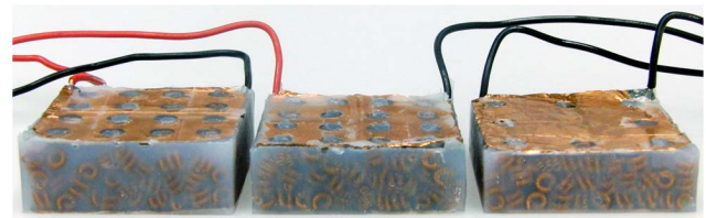
Figure 10. Image of a 300 cell sample of each of the three types of composite. Unjammed: left, Jammed: middle, Jammed, pre-stressed: right. Notice the decreasing height of the samples as the packing fraction increases from Unjammed to Jammed pre-stressed. doi:10.1371/journal.pone.0082260.g010
