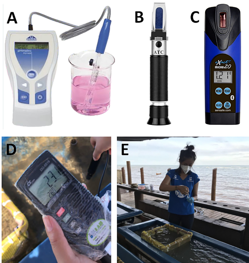
Fig. 6. Daily routine to monitor the physical and chemical parameters of seawater in the marine mesocosm system: (A) portable pH meter (seawater pH measurement); (B) hand refractometer (seawater salinity measurement); (C) portable multiparameter ( in loco seawater Fe concentration measurement); (D) portable digital dissolved oxygen meter (seawater dissolved oxygen content measurement); (E) seawater samples collection for laboratory quantification of total and dissolved Fe concentrations by Inductive Coupled Plasma Mass Spectrometry (ICP-MS).
