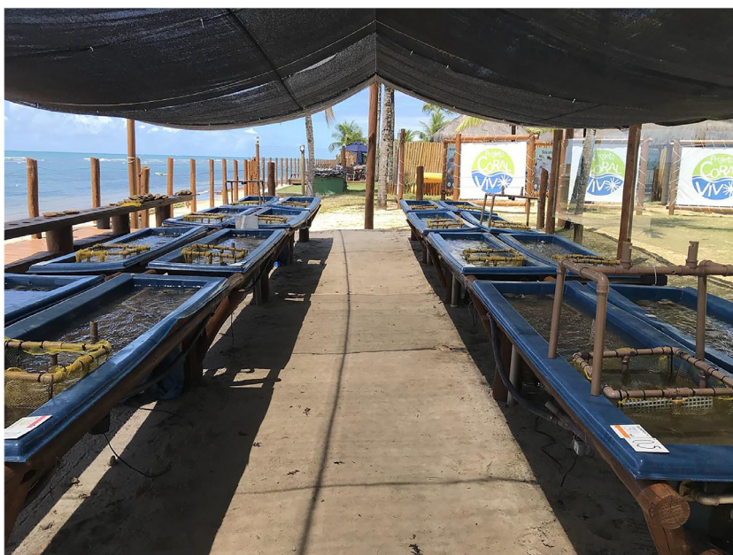
Fig. 3. Sixteen plastic raceways (100×40×30 cm, length x width x height; 130 L) where organisms to be tested are randomly housed according to the control and the desired experimental conditions. Therefore, each experimental condition is run in quadruplicate (4 troughs per experimental condition).
