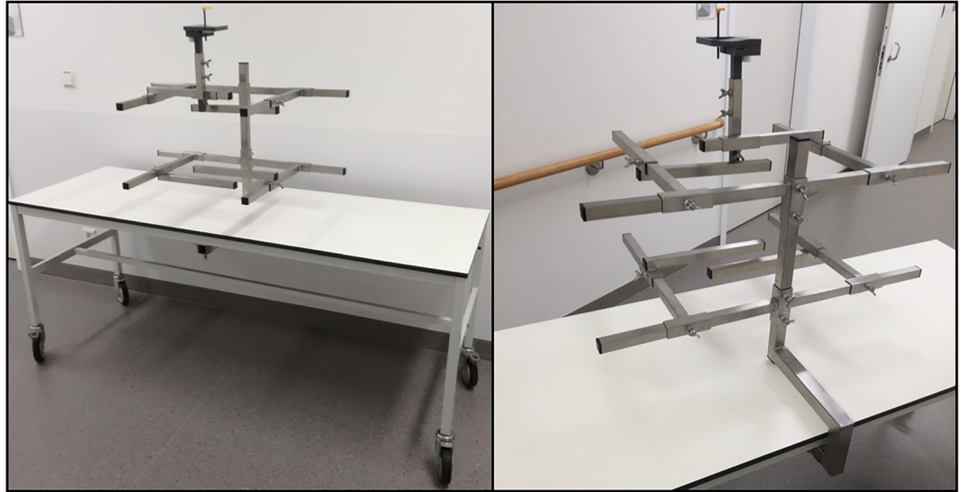
Figure 5. A fixation system developed for post-mortem DPR acquisitions. The upright and the holding arms can be adjusted so that both tall and short bodies can be fixed reliably. A chin rest helps to correctly position the head.
