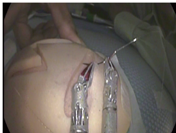
Fig. 1. Master and slave transluminal endoscopic robot suturing with adjustability and versatility in a dry setting.
