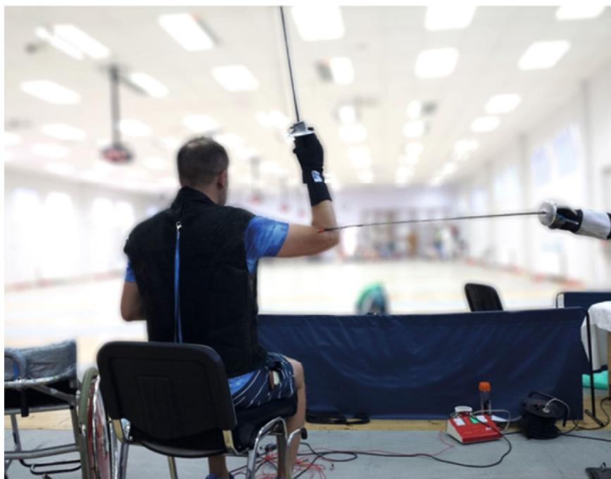
FIGURE 1: Adjustment of fencing piste—distance between the tip of the fencer's weapon and coach's elbow and accelerometer located on the guard of the coach's weapon.
