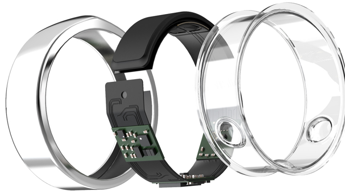
Figure 1. Technical illustration of the second generation Oura ring. The ring has a titanium cover, battery, power handling circuit, double core processor, memory, two LEDs, a photosensor, temperature sensors, 3-D accelerometer, and Bluetooth connectivity to a smartphone app.
