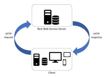
Figure 4. REST API synchronous communication schema.
