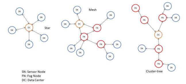
Figure 2. Star, mesh and cluster-tree architecture schema.
