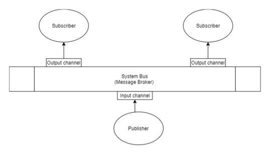
**Figure 5.** Publisher-subscriber architecture based on asynchronous communication of services interplatform.
