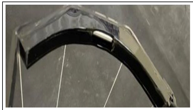
Figure 5. Placement of DS18B20 inside the face shield for the measurement of body temperature.
