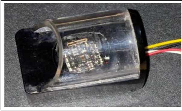
Figure 3. Placement of MAX30102 sensor within the finger clipper that aids in measuring the SpO 2 .
