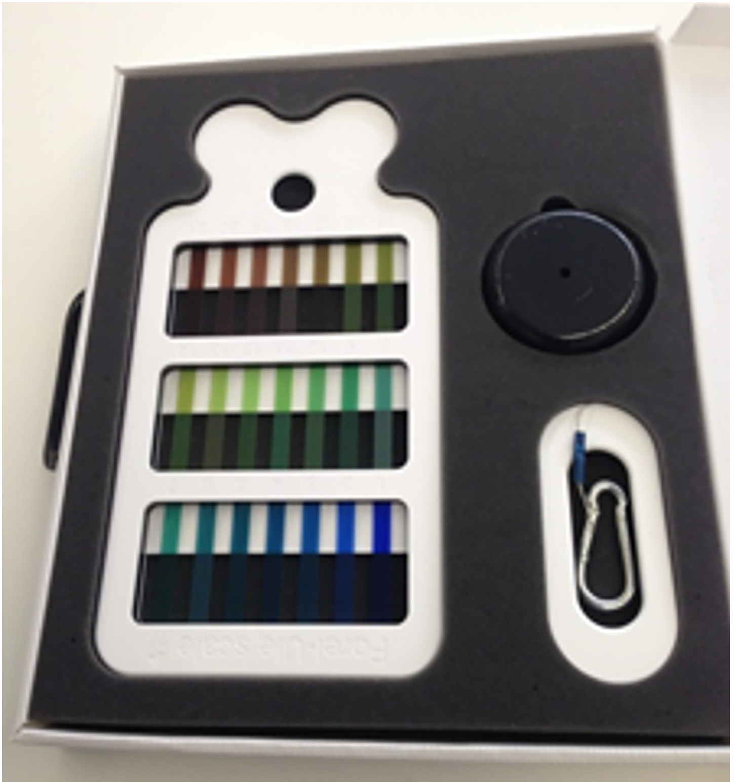
Fig 9. The “Modern Forel-Ule scale” using plastic colour filters, together with a Secchi disk.
