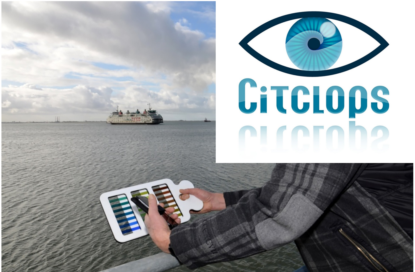
Fig 10. The “Modern Forel-Ule scale” using plastic colour filters.
