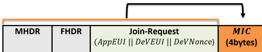
Figure 3. The Join-Request message structure.
