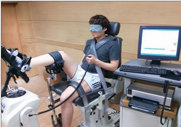
Figure 3. Measurement of Joint Position Sense on Ankle (Biodex system 4pro, Biodex medical systems, Inc., USA).
