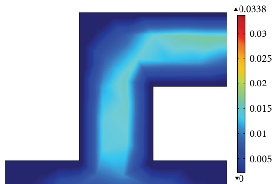
FIGURE 8: Schematic presentation of velocity flow at sharp corner of microfluidic channel.
