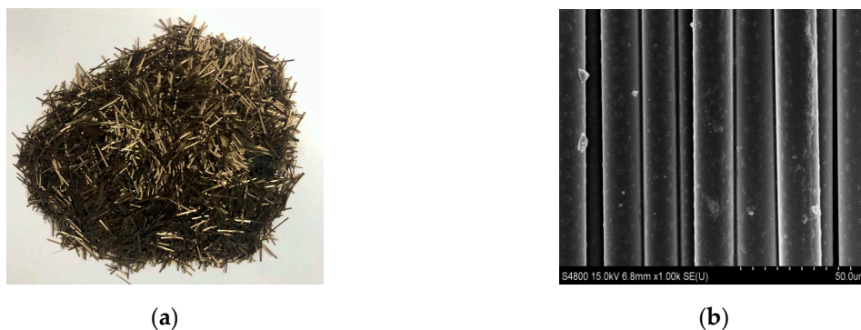
Figure 1. Morphologies of basalt fiber: (a) appearance; (b) scanning electronic microscope image.
