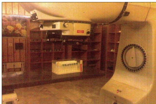
Figure 2: Irradiation of samples in tissue equivalent phantom
