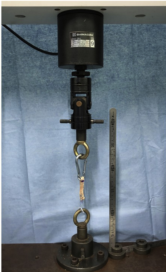
Fig 4. The specimen was mounted on a universal material testing machine. The free strands of suture were tied to a hook 20 mm from the tendon end.
