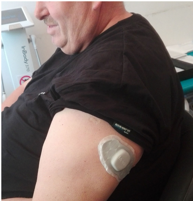
Fig. 1 Metria IH1 device that continuously measures physical activity over 1 week
