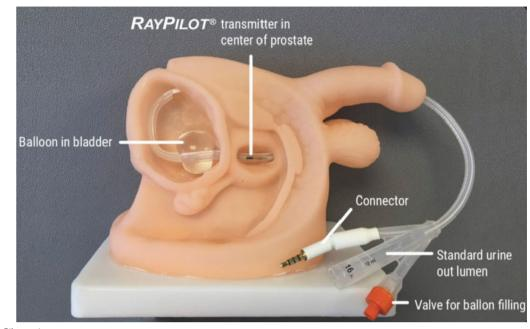
Fig. 1 RayPilot main components
