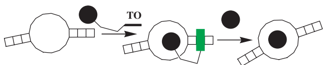
Scheme 1. Principle behind light-up probes for aptamers and their displacement with unconjugated small molecules: An RNA aptamer against a molecule (circle) binds a conjugate between molecule and TO dye, resulting in a fluorescent complex. Presence of free molecule in solution results in displacement of conjugate from the complex and reduction in fluorescence.
