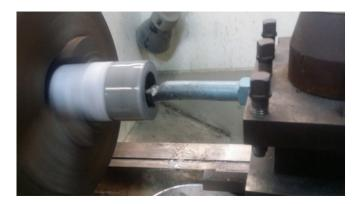
Figure 3. Wet drilling the binding samples using a lathing machine.
