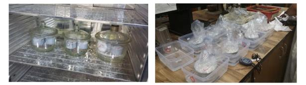
Figure 2. Sorptivity conditioning in KBr (left) and sorptivity testing setup (right).
