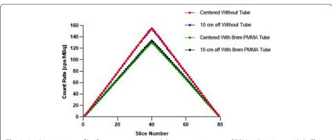
**Fig. 2** Axial sensitivity profiles for measurements with line source in center of FOV and at 10-cm radial offset with or without 8 mm thickness PMMA tube
