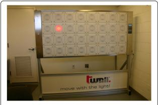
Fig. 3 The t-wall. The participant goes through a random sequence of striking 100 lighted buttons, one immediately after the other
