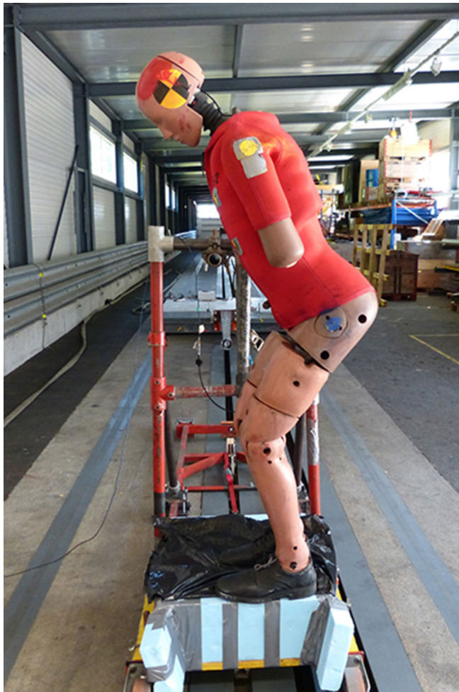
Figure 2 Dummy positioned on the sled in the upright position. The different targets and markers on the dummy were used to verify that the same position was used in every test.
