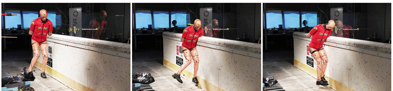
Figure 3 Example of impact tests with the ES-2 crash test dummy. (Left) Sled motion was stopped abruptly; (middle) dummy slides off the sled towards the board in an upright position and (right) dummy position on impact.
