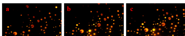
Figure 17. Emulsification for 17 (a), 51 (b), and 120 min (c) of oil sample A after evaporation for 120 h.
