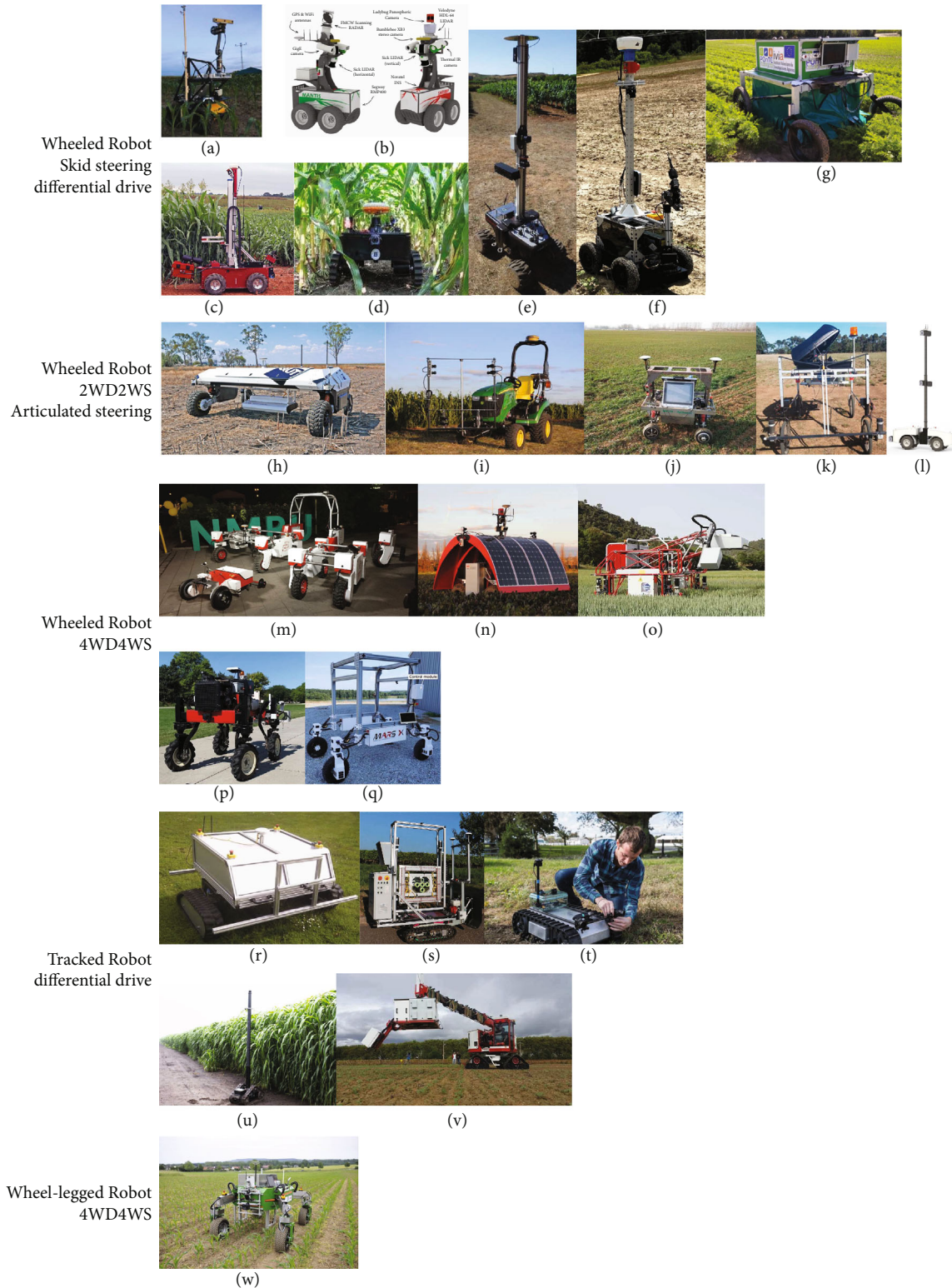
FIGURE 2: Phenotyping robots. (a) Vinobot [24]. (b) Shrimp [25]. (c) Robotanist [26]. (d) TerraSentia [27]. (e) VinBot [28]. (f) MARIA [29]. (g) RobHortic [30]. (h) AgBotII [31]. (i) Phenobot 1.0 [32]. (j) AgriRover-01 [33]. (k) DairyBioBot [34]. (l) Phenobot 3.0 [35]. (m) Thorvald II [36]. (n) Ladybird [37]. (o) Phenomobile V1 [38]. (p) Flex-Ro [39]. (q) MARS X [40]. (r) Armadillo Scout [41]. (s) PHENObot [42]. (t) A robot based on LT2 [43]. (u) TERRA-MEPP [44]. (v) Phenomobile V2 [45]. (w) BoniRob [46].
