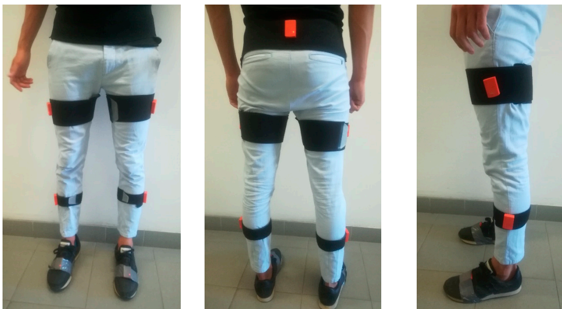
Figure 1. Example of IMU (inertial measurement unit) placement on lower limbs of one subject: frontal, back, and lateral view.
