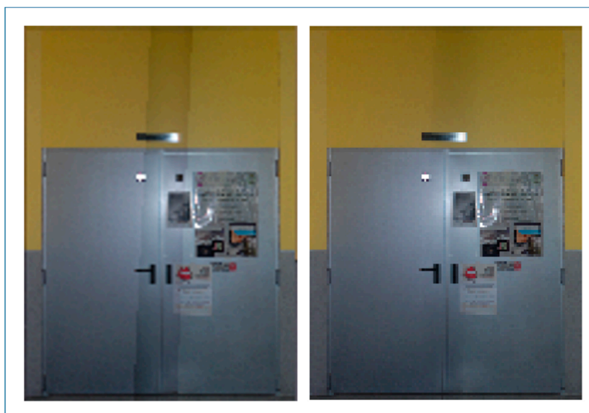
Figure 14. Left orthoimage presents edge seams as opposed to right orthoimage, where pixels are fused making the overlapping area transitioned from the first image to the second image slowly.
