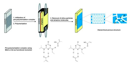
**Figure 8.** Schematic illustration of the procedure used for the preparation of the molecularly imprinted photonic polymer. Reproduced with permission from [32].
