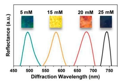
**Figure 12.** Red shift in peak optical reflectance of hydrogel-encapsulated CCAs with increasing concentration of immobilized negatively charged groups from phosphorylation of peptides (at pH 5.5). Reproduced with permission from [26].
