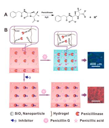
**Figure 13.** (A) Enzymatic reaction between penicillinase and penicillin G; (B) Schematic illustration of the PCCH (penicillinase colloidal crystal hydrogel) sensor for the detection of  $\beta$ -lactam antibiotic and  $\beta$ -lactamase inhibitor. Reproduced with permission from [41].
