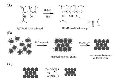
**Figure 6.** (**A**) Synthesis of HEMA-modified microgels by coupling of P(NIPAm-AAc) microgels with HEMA under catalysis by EDC. (**B**) Synthesis of polymerized microgel colloidal crystals (PMCC). (**C**) Response of PMCC to temperature or salt. Note: HEMA: 2-hydroxyethyl methacrylate; AAc: acrylic acid; EDC: *N*-(3-dimethyla-minopropyl)-*N*'-ethylcarbodiimide hydrochlorid. Reproduced with permission from [30].
