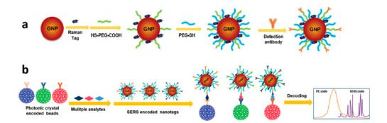
**Figure 14.** Schematic of the SERS nanotag preparation (**a**); and multiplex bioassays encoded by photonic crystal beads and SERS nanotags (**b**). Reproduced with permission from [42].
