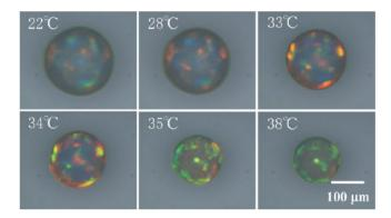
**Figure 3.** Photographs of the reflection at normal incidence of a thermosensitive PNIPAm-immobilized colloidal crystal sphere at various temperatures. Reproduced with permission from [27].
