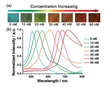
**Figure 9.** (a) The colorimetric transition of the molecularly imprinted polymer-photonic crystals dot as the tetracycline concentration increasing. (b) The spectra with different concentrations dried on MIP-PC dots with a diameter of 1.35 mm. Reproduced with permission from [33].
