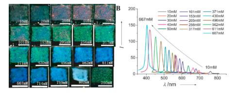
**Figure 7.** (**A**) Photographs of a freestanding PMCC film taken with [NaCl] increasing from 0 to 750 mM. The last one (bottom right) was taken when [NaCl] was decreased back to 250 mM. Scale bar: 0.5 cm. pH 3.0. T = 238 °C. (**B**) Reflection spectra of the PMCC film measured at various [NaCl] values. Reproduced with permission from [30].
