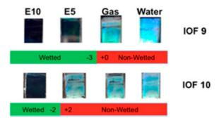
**Figure 4.** Optical images show the wettability tests on the coated IOF strips when dipped in gasoline/ethanol mixtures. Reproduced with permission from [28].
