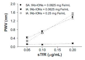
**Figure 17.** Comparison of linear responses when using inverse sandwich assay (IA) at 0.0625 and 0.25 mg Fe/mL with the standard assay (SA) at 0.0625 mg Fe/mL to measures transferrin receptor (TfR) on the 3DOCs biosensor. Iron-oxide nanoparticles with antibodies: fAb-IONs. PWV: peak shift. Responses were measured at 200 min. Reproduced with permission from [44].
