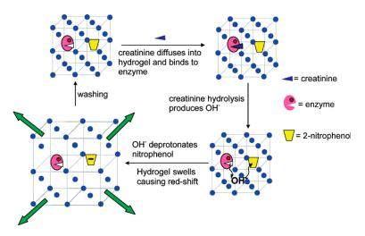
Figure 10. Schematic depiction of the creatinine sensor concept. Reproduced with permission from [39].
