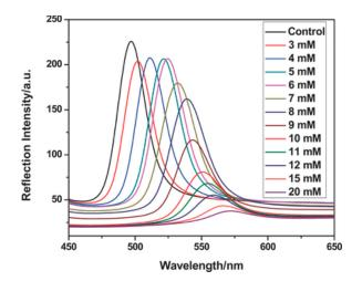
**Figure 2.** Optical responses of PNA OCP PC to different glucose concentrations. Note: PNA: MMA–NIPA–AAPBA; OCP: opal closest-packing; PC: photonic crystal. Reproduced with permission from [26].
