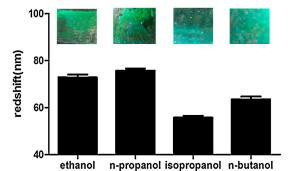
**Figure 5.** The red shift and structural color of 3DOCs in different alcohols. Reproduced with permission from [29].
