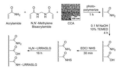
**Figure 11.** Fabrication of a Kinase Responsive CCA (crystalline colloidal array) Biosensor. Reproduced with permission from [40].
