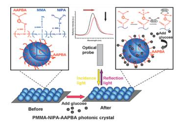
**Figure 1.** Experimental procedure for the reflectometric glucose detection using microsphere-based 3DOCs. Reproduced with permission from [26].
