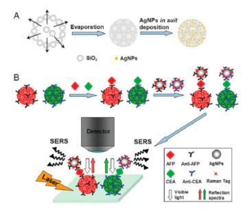
**Figure 16.** The schematic illustration of the fabrication of Ag-SPCBs (silver nanoshells silica photonic crystal beads) (**A**); and the multiplex SERS bioassay (**B**). Reproduced with permission from [43].
