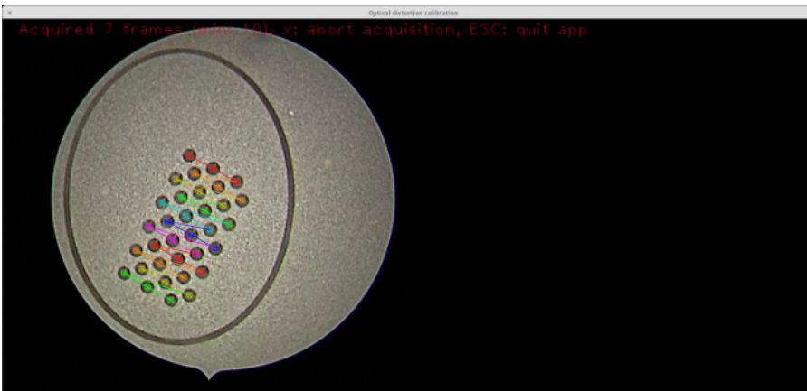
Figure 3: Real-time detection of the calibration pattern. A screenshot from the calibration application 16 featuring the detected calibration pattern overlaid onto the live video stream using the virtual reality visualization from OpenCV 17 . Note that each detected column of the calibration pattern is emphasized by a different color. The detected circles, in conjunction with the known geometry, are used for computing the camera parameters. Please click here to view a larger version of this figure.
