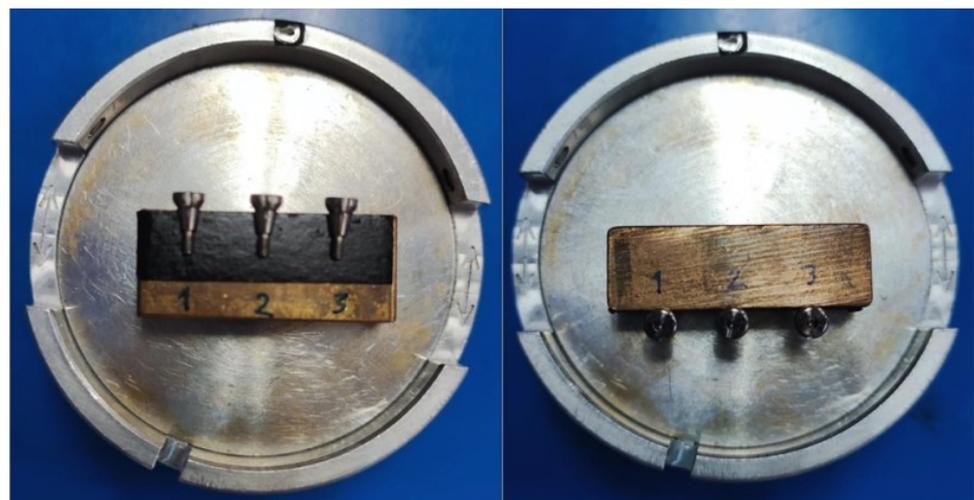
**Figure 3.** Sample preparation for the scanning electron microscope (SEM).
