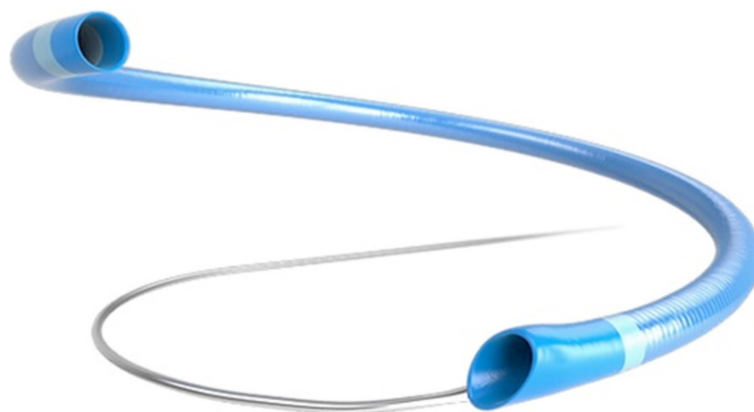
Figure 1. The MIVI Q system consists of a distal catheter with a flared proximal end that forms a tight seal with the selected guide catheter, and a proximal stainless steel wire replaces the proximal shaft of a traditional catheter design.
